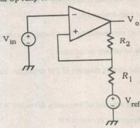
Show that  $V_{TU} = V_C + V_H \frac{R_1}{R_1 + R_2}$
